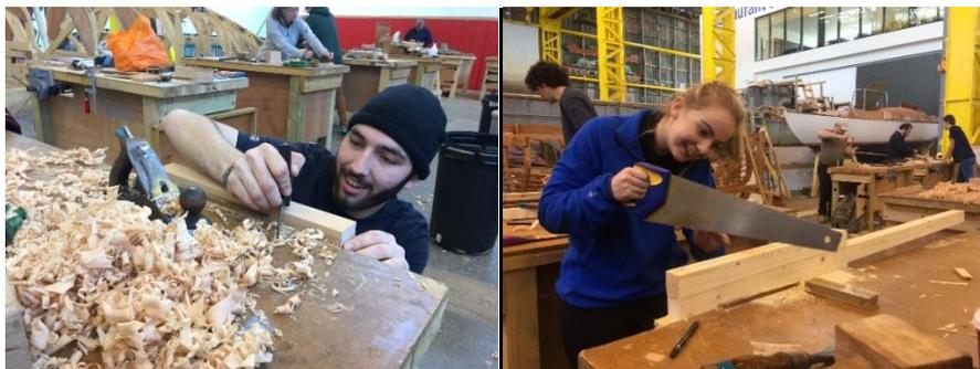
*Fig. 4: Wood working with traditional tools to make a mallet (left) and a paddle (right).*
