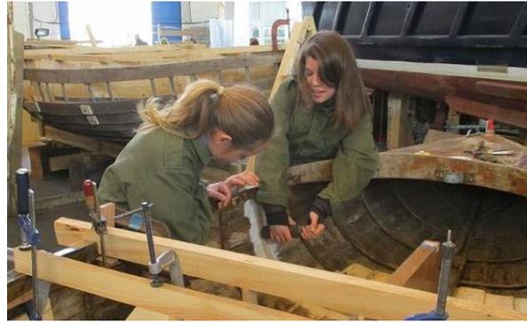
*Fig. 6: Installing a steam-bent rib.*
