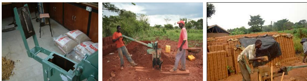
Figure 1: Interlocking Stabilised Soil Block (ISSB) using a Makiga Ram
