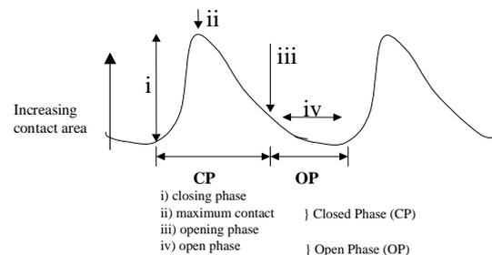
Fig. 1 Idealised electrolaryngograph output waveform (from [4:206])
