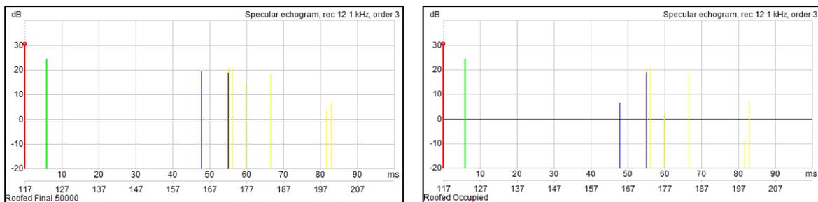
Figure 3: Energy of Specular Reflections. EHA (left) & OHA (right)
