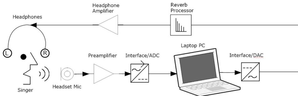
Figure 1: Recording setup
